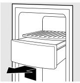
Pull the bin straight out, then lift past the **stop** position.
